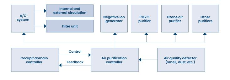
Figure 15 Reference architecture for the Indoor Air Quality Assurance System
