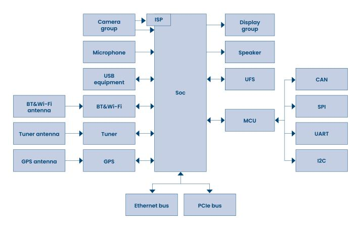
Figure 7 Reference architecture for the cockpit domain controller system
