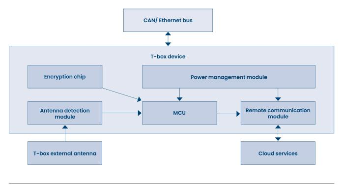
Figure 14 Reference architecture of the T-box system
