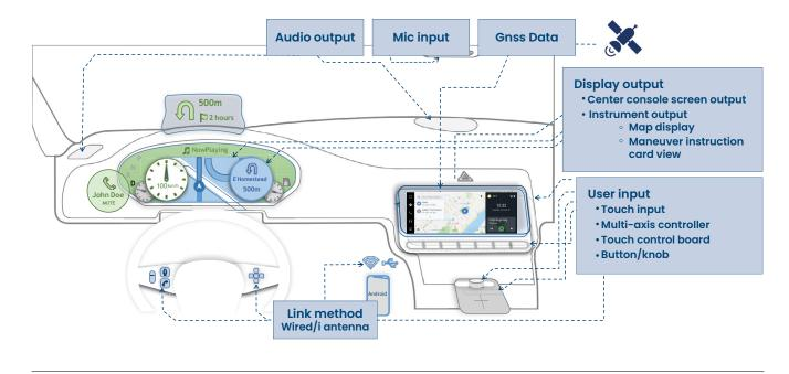
Figure 21 Principles of mobile phone screen projection technology
