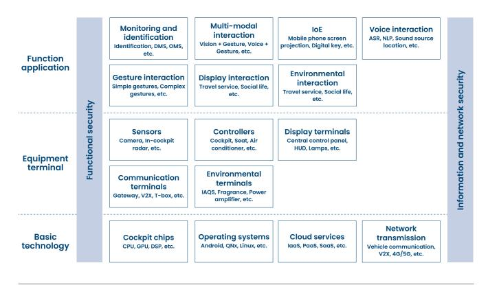
Figure 3 Reference architecture for the intelligent cockpit
