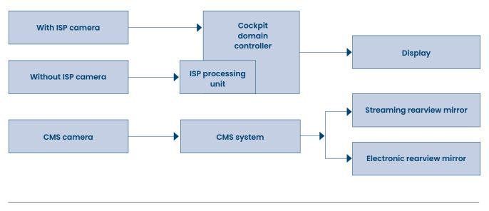
Figure 5 Reference architecture for a cockpit camera system
