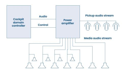
Figure 17 Reference architecture for the auto audio system (both internal and external power amplifiers are applicable)
