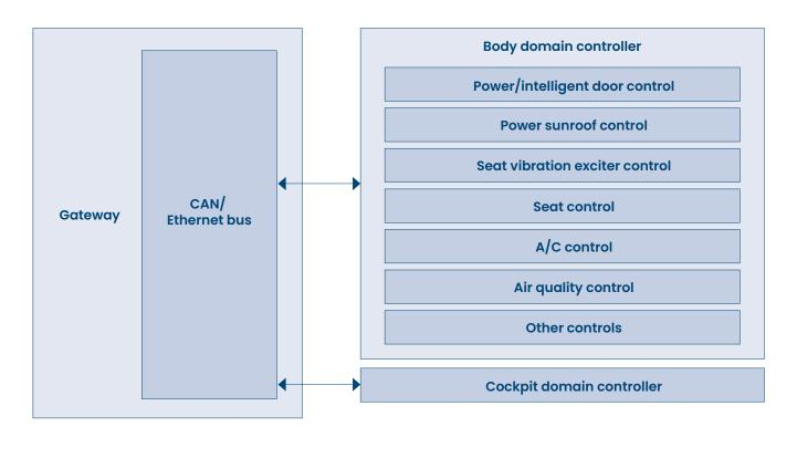
Figure 9 Reference architecture for the centralised body control system
